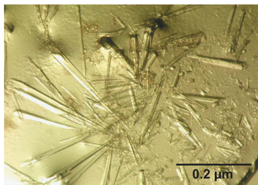
Figure 2 Crystals of Lv -ranaspumin grown by the sitting-drop vapour-diffusion method at 293 K in 0.2 M KCl, 20% (w/v) PEG 3350 pH 7.0.
